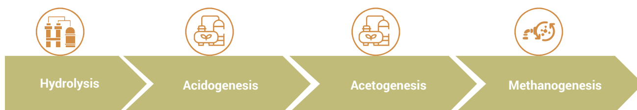
Figure 6: Bio-chemical Process Flow for Biogas Production
