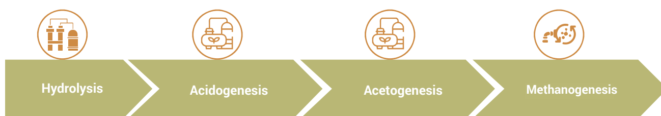
Figure 6: Bio-chemical process flow for biogas production
