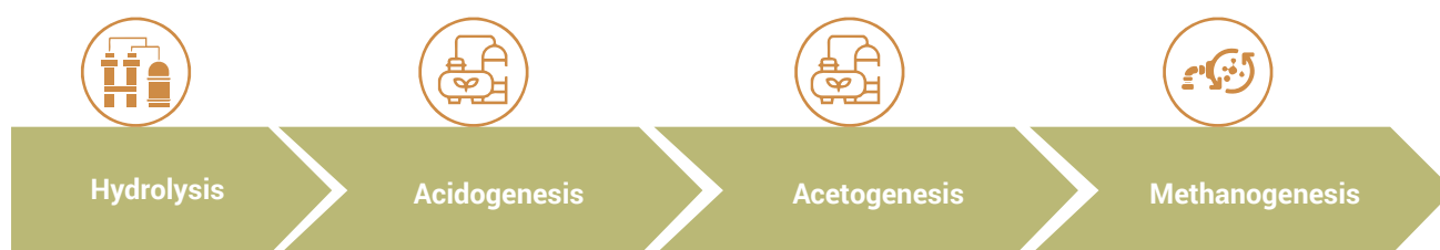
Figure 6: Bio-chemical process flow for biogas production
