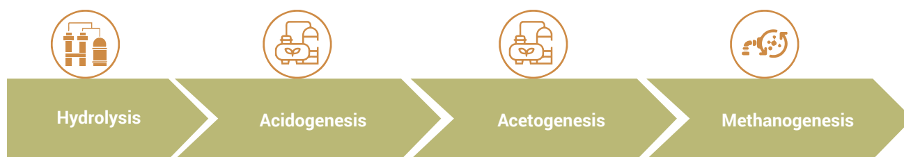
Figure 6: Bio-chemical process flow for biogas production
